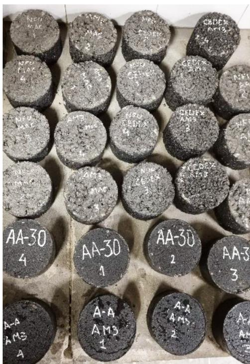
Figura 7: Probetas Marshall
