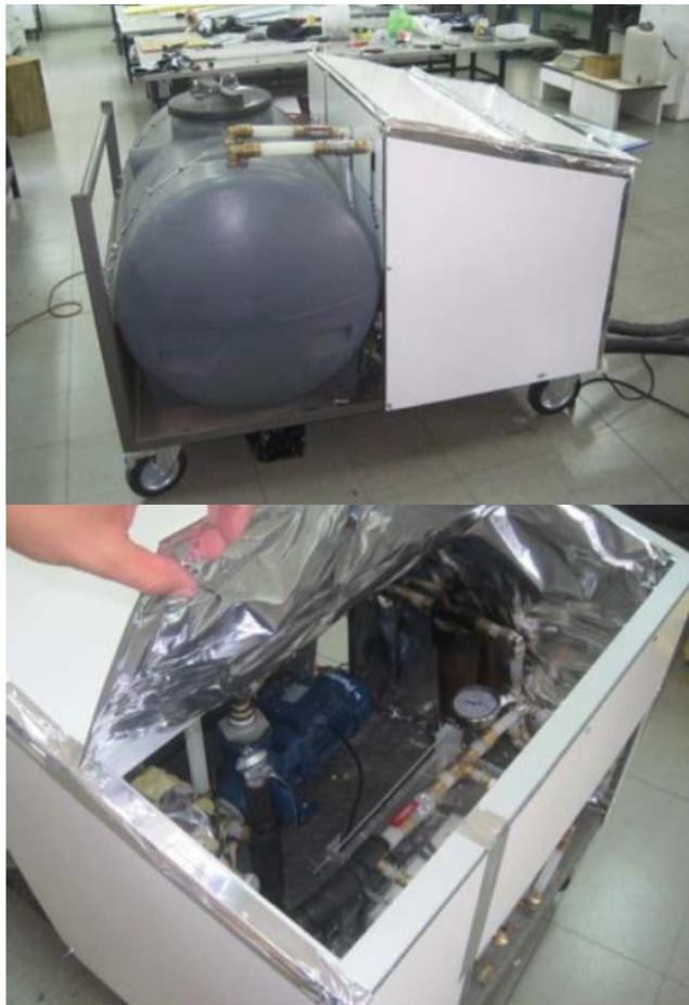
Figure 8: TRT equipment built for this research
